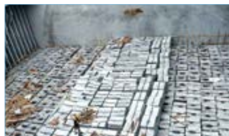
Lashing and chocking with adequate fumigated dunnage inside vessel hold to avoid metal-to-metal contact
