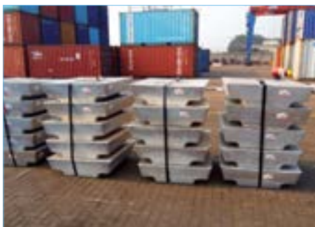
Unitisation of bundles using industrial-grade straps and cargo stacking at yard
